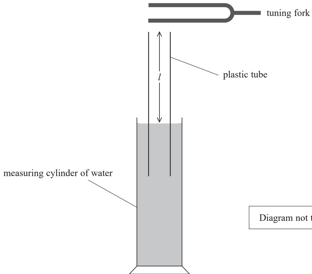
The student adjusted  $l$  until the loudest sound was heard, indicating that a standing wave had formed. He marked the water level on the plastic tube and measured  $l$ .
